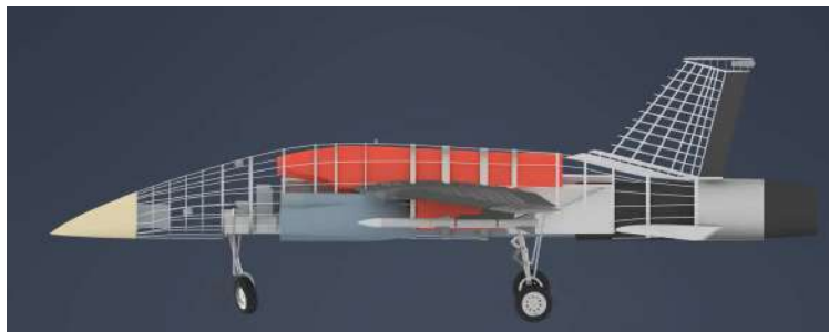
Fig. 62 Image of the landing gear during retraction at point of nose gear rotation.
